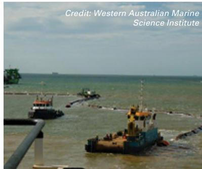
▲ Vessels connecting discharge pipeline from cutter suction dredge to hopper barge at Wheatstone. This is part of the day-to-day activities of the Dredging Science Node, which is one of the largest single-issue marine research programs in Australia.
