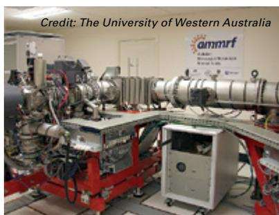
▲ The CAMECA IMS 1280 (located at the Centre for Microscopy and Characterisation) is a versatile member of the latest generation of double focusing, magnetic-sector SIMS instruments.
